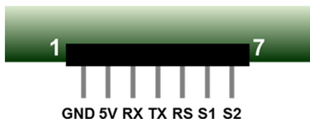
FIGURE 14 – 7-pin header, showing the function of each pin
